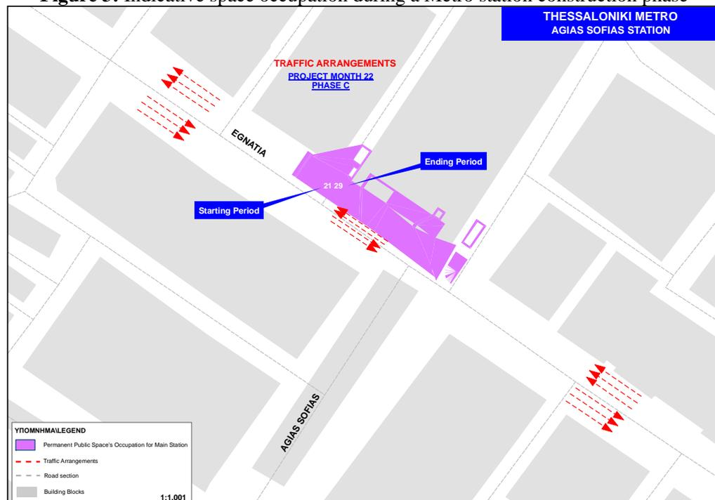
**Figure 4:** Indicative space occupation during a Metro station construction phase (differentiation from Figure 3)
