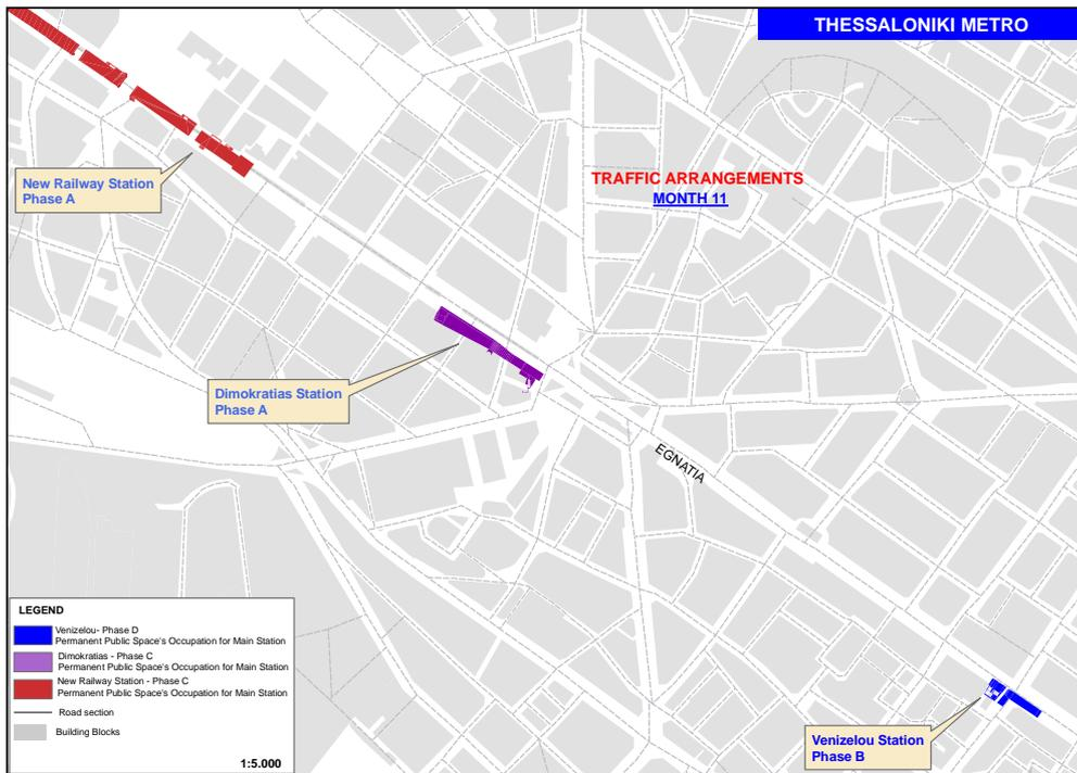
**Figure 6:** Indicative space occupation for the 11<sup>th</sup> month of Metro construction over the area of three Metro stations
