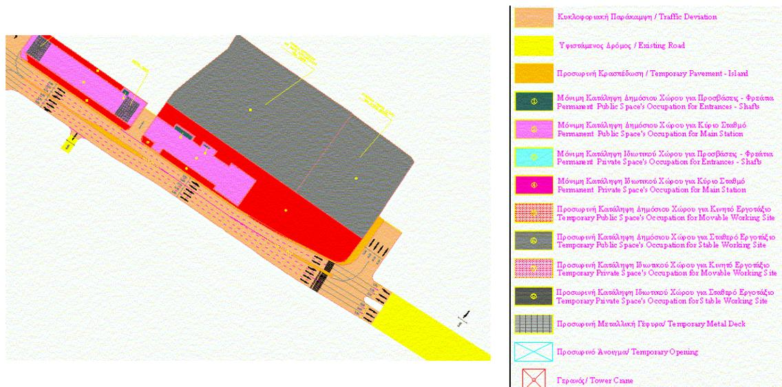
**Figure 1:** Indicative space occupation during a metro station construction phase
