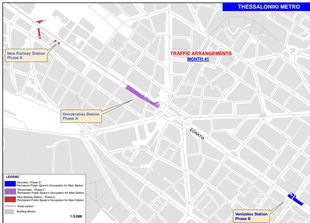
**Figure 7:** Indicative space occupation for the 41<sup>st</sup> month of Metro construction over the area of three Metro stations
