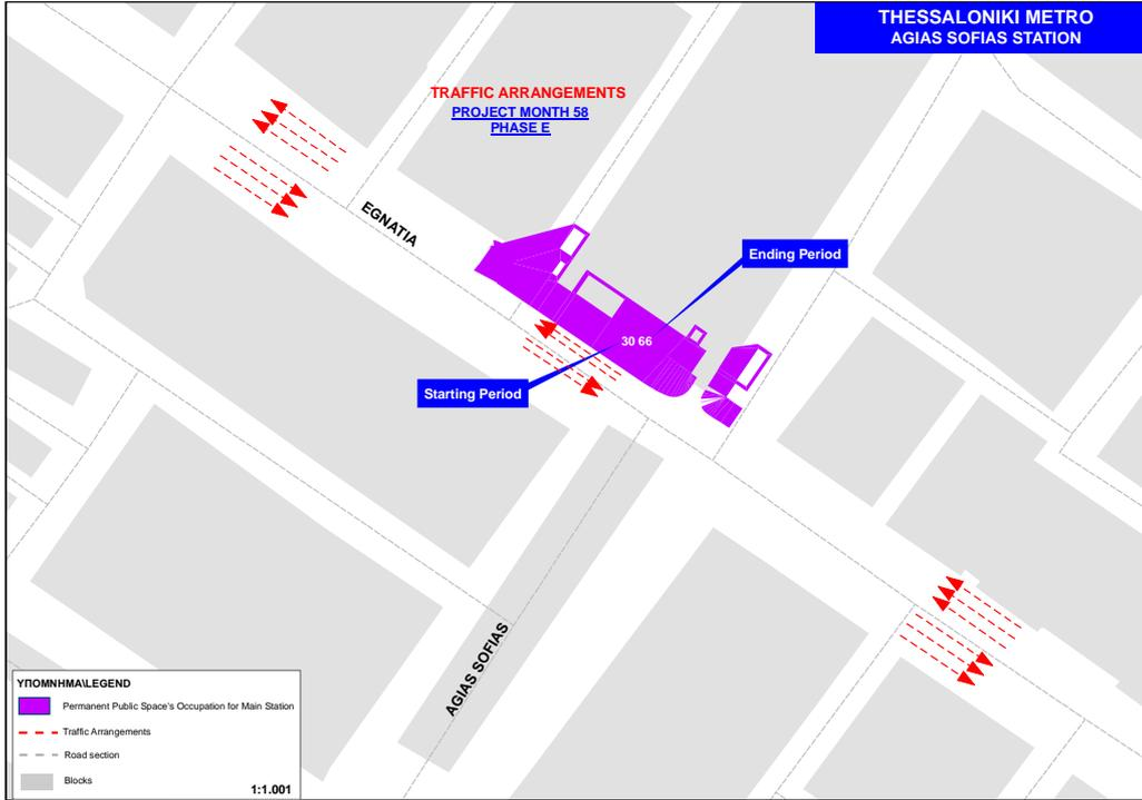
**Figure 5:** Indicative space occupation during a Metro station construction phase (differentiation from Figures 3 and 4)
