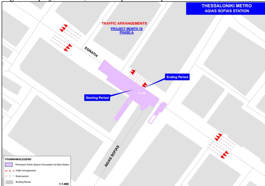
**Figure 3:** Indicative space occupation during a Metro station construction phase
