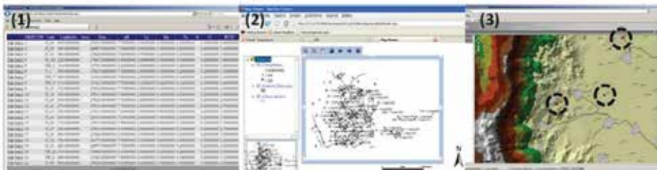
Fig. 3. Ground water information management system: (1) data input; (2) sampling points; (3) alarm (highlighted points in dotted circles) on exceedance of user defined threshold
